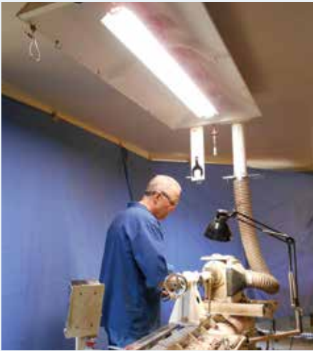
Bob Rosand's lighting at the lathe includes both an overhead LED tube fixture and an adjustable task light.
